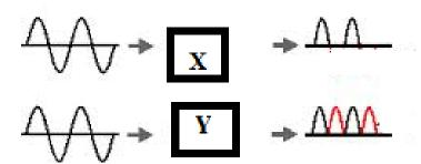
b) If the frequency of the input signal is 50Hz, what will be the frequency of the output signal in X & Y.
